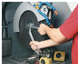
Easy Exchange of Cut Off Wheel
