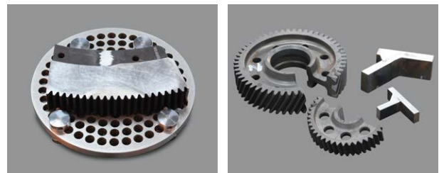
Ability to grind mounted specimens with specimen holders as well as irregular shaped unmounted samples.
